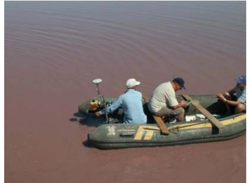
Echo sounding at El Jem: system configuration. The GPS antenna is clearly visible
